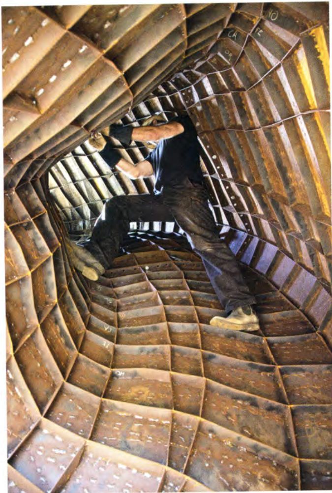
(l) Welding inside the Rex Australis and (above) the whole sculpture is fabricated from thousands of small, flat Corten steel plates. (r) Halo stands tall in newly established parkland in Chippendale, Sydney.
